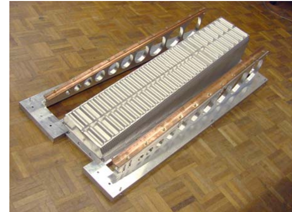
Prototype of the secondary vacuum box and RF foil
