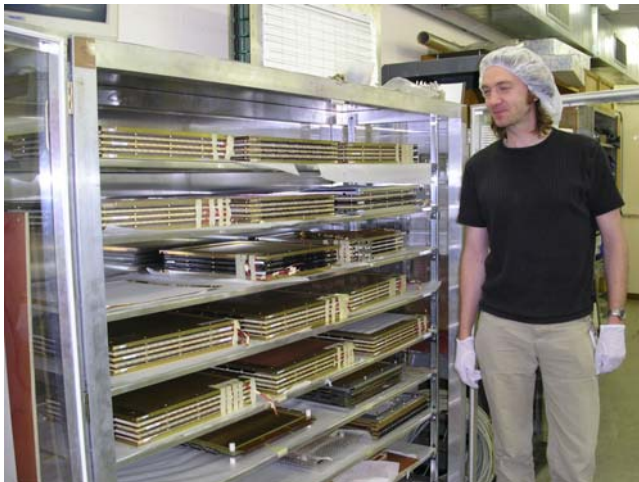
Inner chambers of station M3
