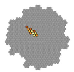
Once detected by the telescope's camera the light results in an "image" of the corresponding air shower event
