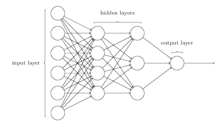
Artificial neural network is a mathematical object represented by nodes, arranged in layers. An output of a node is a result of an activation function applied to a linear combination of input "signals", with weights associated with each input.
